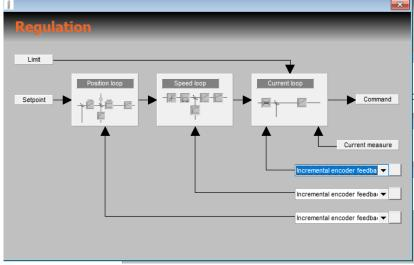
Set the associated feedback of each loop (Current, Speed, position). In our case, all value are get with the same incremental feedback.
